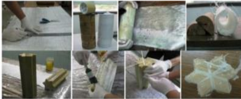
Figure 10 Hand lay-up method
