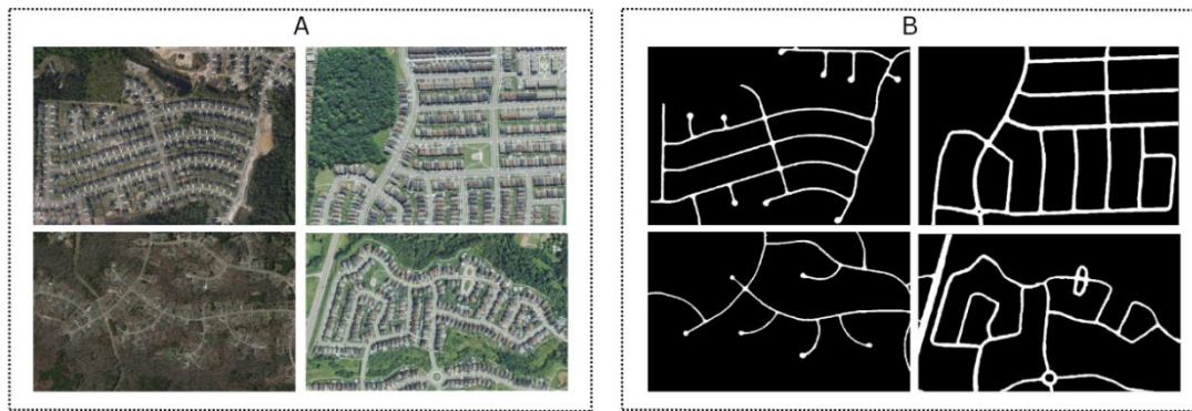
Fig. 1. High resolution satellite images and their corresponding mask (A) training image set (B) corresponding mask to training set
