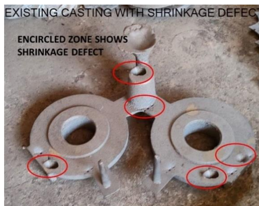
Figure 1 Shrinkage defect in casting
